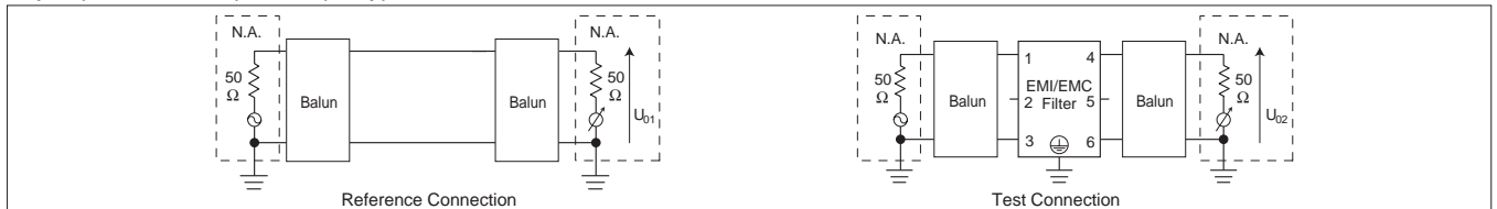
Fig.3.3 Differential mode attenuation measurement diagram
