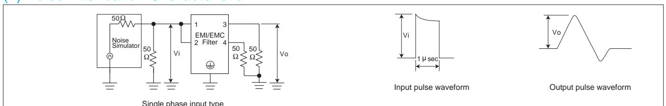
Fig.3.7 Pulse attenuation measurement diagram
