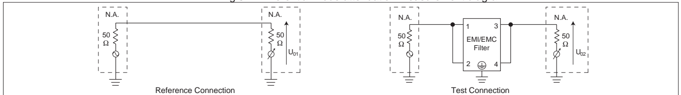
Fig.3.2 Common mode attenuation measurement diagram
